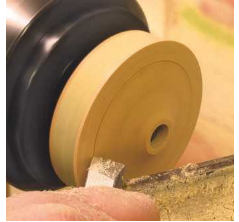
▲ Pic.12 The edge of the top needs to be quite thin, around 2 to 3mm is perfect. He likes to put a little detail on the top and is using the point of a skew to scrape some decorative lines
